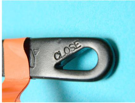
It may take more than one time to close the QR handle to adjust the proper tension. When closed properly the QR Handle should be tight, in the 2-3 o'clock position (pointed back) almost pressed against the fork, locking the wheel tightly in place. This is the same process every time the front wheel is removed or replaced.
