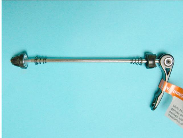
Remove the tightening nut and one spring from the skewer, confirm that remaining spring is wide end out/narrow end contacts axle. Slide skewer into front wheel axle from disc brake side, push all the way in. Place spring on skewer narrow end first. Thread tightening nut onto skewer wide end in, and tighten until several threads show out of the nut opposite end
